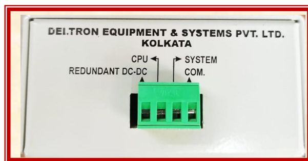
Figure 18:UFSBI Alarm Panel (Back View)
