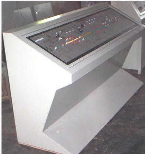
Side view of Control Panel (with provision of Leg space for the operator & faceplate inclination angle of 30°)
