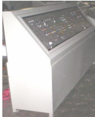
Side view of Control Panel (without provision of Leg space for the operator & faceplate inclination angle of 60°)
