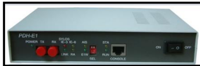
Single Mode OFC to E1 & RS232 (20 Km typically upto 80 Km)
